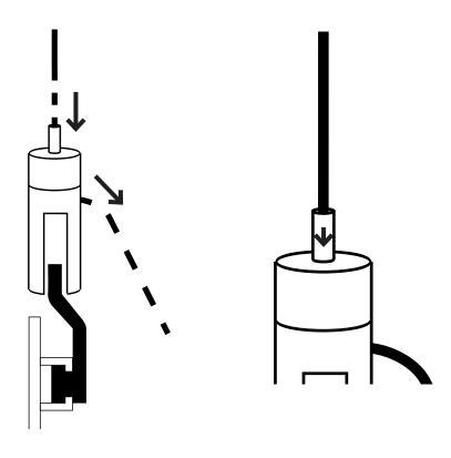
NOTE: If you pull too far the screen can be lowered by pushing down the button on the top of the flying mount.
